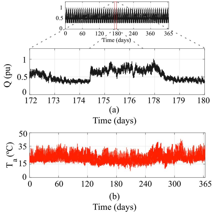
Figure 29 – Mission profiles with a sampling time of 5 min: (a) Reactive Power; (b) Ambient Temperature.
