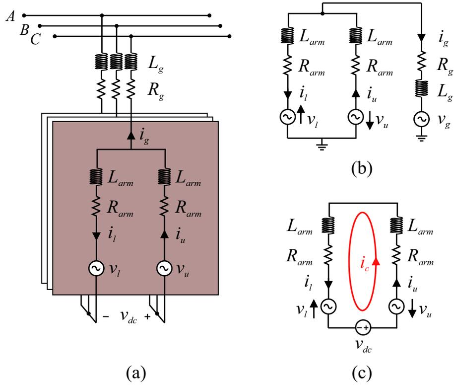
Figure 10 – Schematic of the DSCC-MMCC-based STATCOM: (a) Average model; (b) Equivalent circuit describing the output current dynamics; (c) Equivalent circuit describing the circulating current dynamics.
