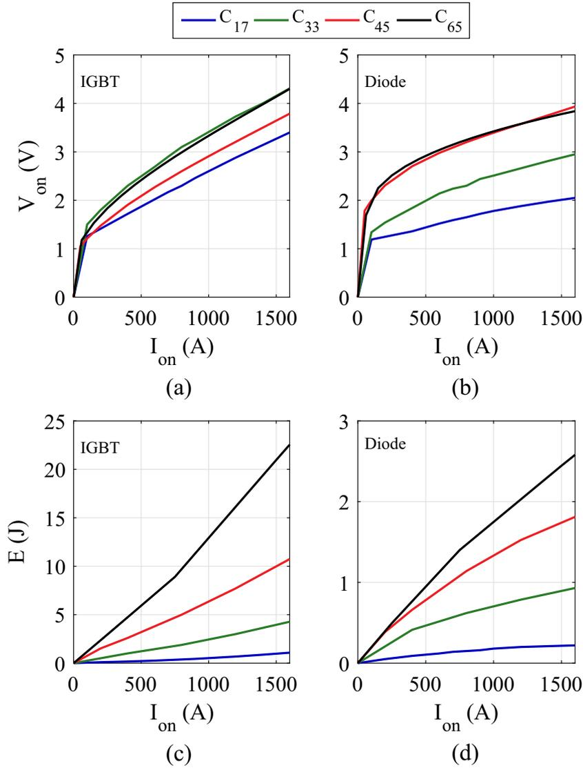
Figure 30 – Typical power devices curves extracted from datasheets: (a) IGBT on-state characteristics; (b) Diode forward characteristics; (c) IGBT switching energies per pulse; (d) Diode reverse recovery characteristics.
