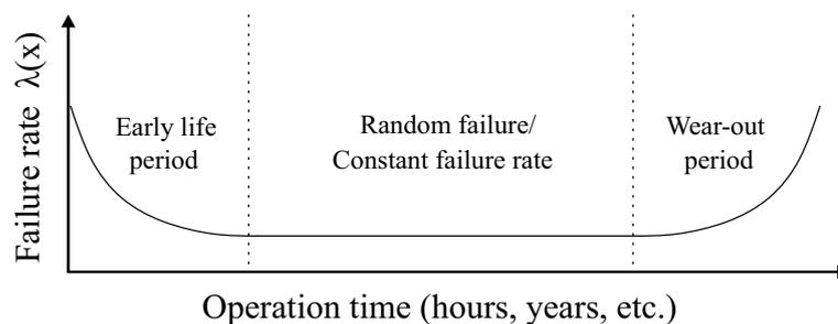
Figure 21 – Typical failure rate curve - bathtub curve.
