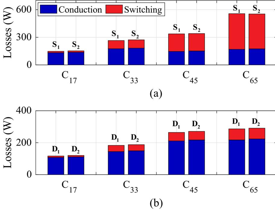
Figure 32 – Power losses for all cases of power devices: (a)  $S_1$  and  $S_2$ ; (b)  $D_1$  and  $D_2$ .
