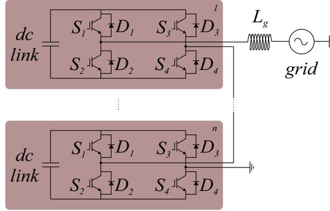
Figure 5 – Single-line diagram of  $(2n+1)$  level CHB.
