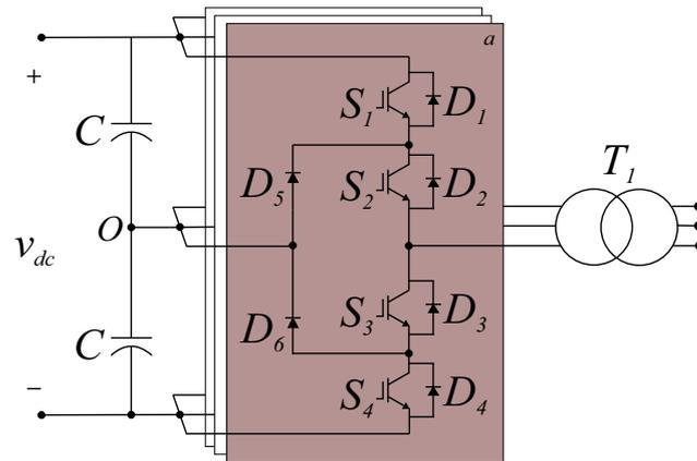
Figure 4 – Three-phase three-level NPC converter with step-up transformer.
