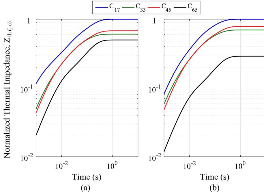
Figure 31 – Normalized transient thermal impedance characteristics for all cases: (a) IGBT; (b) Diode.
