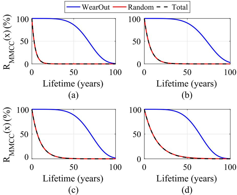
Figure 36 – MMCC system-level reliability-based on wear-out and constant failure rates contributions factors and the total converter reliability: (a)  $C_{17}$ ; (b)  $C_{33}$ ; (c)  $C_{45}$ ; (d)  $C_{65}$ .
