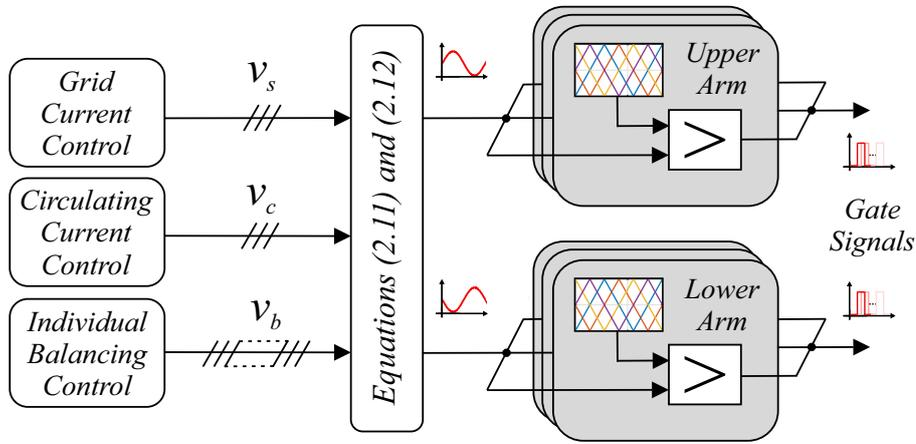
Figure 13 – Connection between the control and the modulation scheme.
