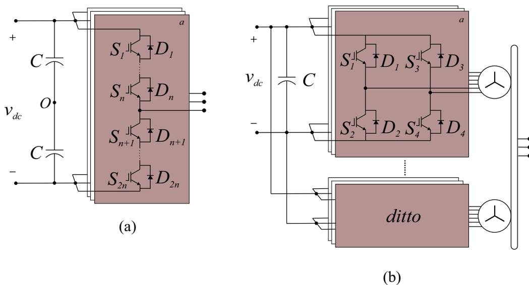
Figure 3 – Two-level voltage source converter: (a) with series connection of semiconductor switches; (b) with a Multi-Stage Transformer.
