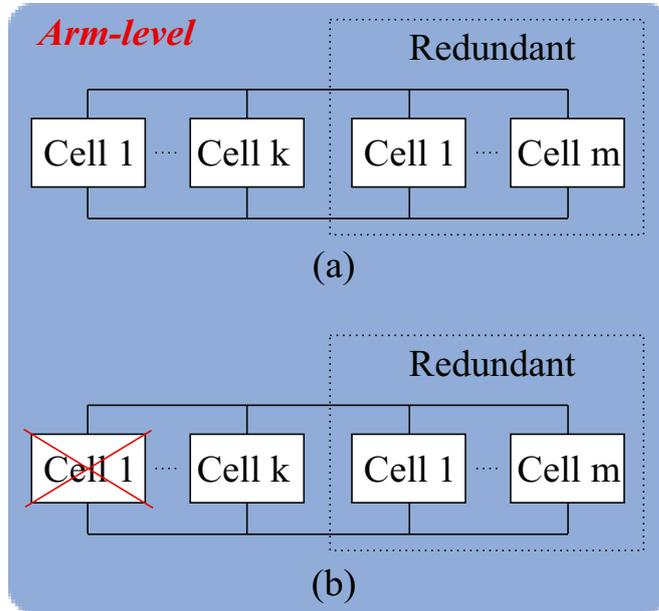
Figure 39 – Arm-level reliability block diagram of MMCC considering redundant cells: (a) without cell failure; (b) with one cell failure.
