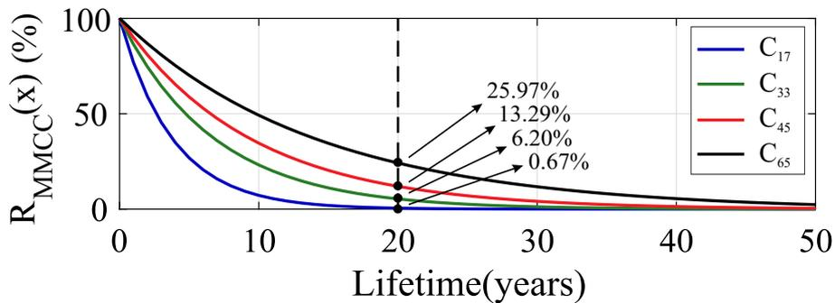
Figure 37 – MMCC system-level reliability function for different solutions.
