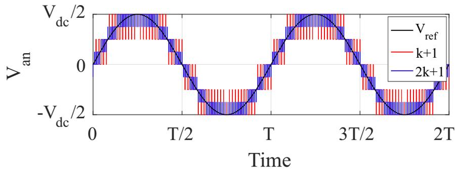
Figure 12 – DSCC-MMCC output voltage comparison of  $(k+1)$  level and  $(2k+1)$  level phase-shifted modulation schemes. *Remark:*  $k = 4$  cells per arm.
