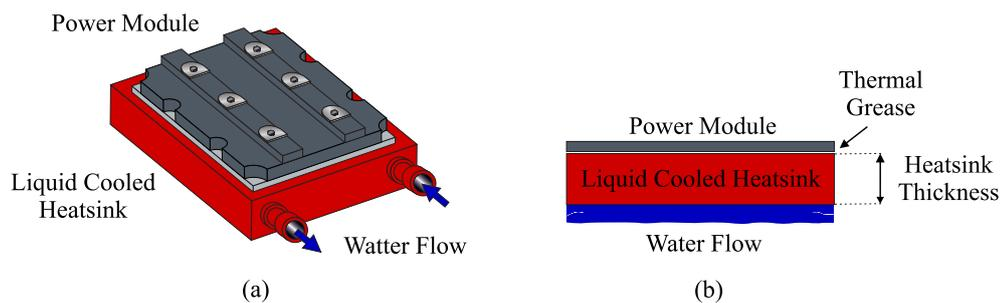
Figure 25 – Heatsink scheme of the water cooling system: (a) Detailed view; (b) Simplified model. Adapted from (Júnior et al., 2019).
