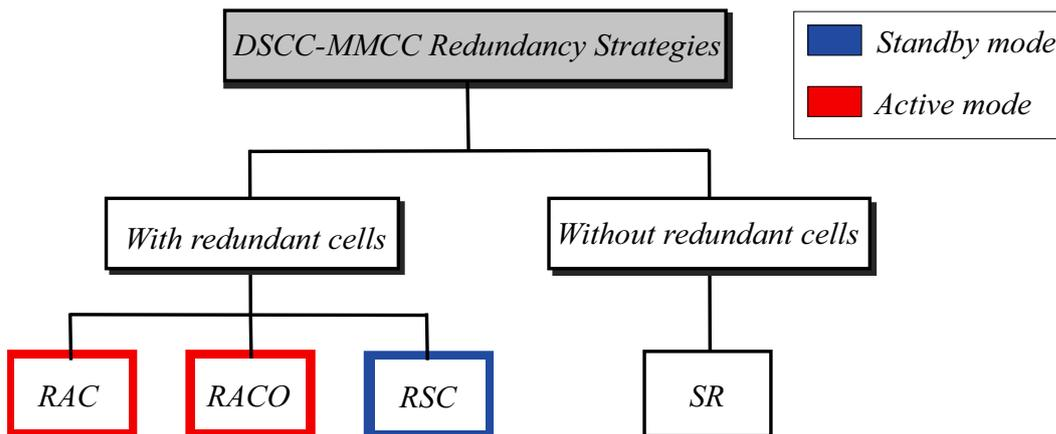
Figure 38 – Classification of the DSCC-MMCC redundancy strategies.
