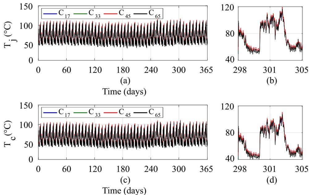
Figure 34 – Temperatures of the more stressed device  $D_2$  in a cell for four designs: (a) Junction temperature; (b) Detailed view of (a); (c) Case temperature; (d) Detailed view of (c).
