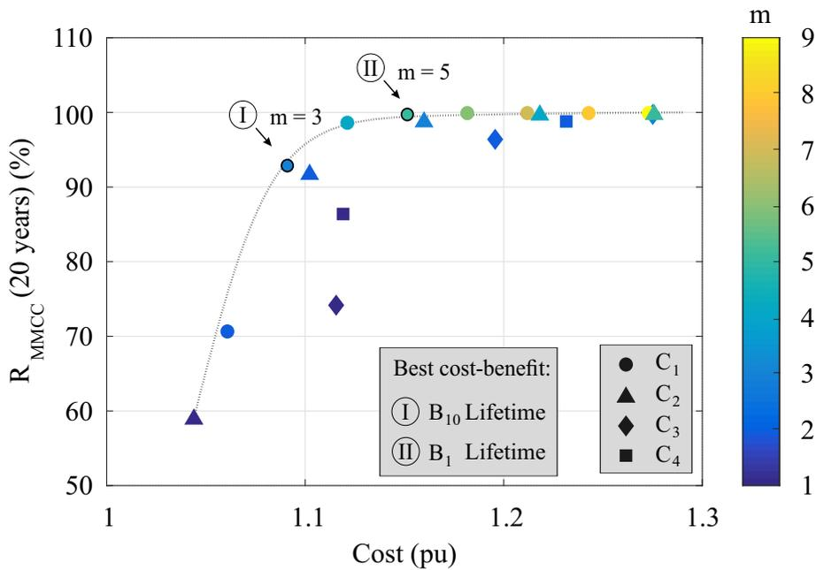
Figure 44 – *Reliability vs cost* of all MMCC solutions for different redundancy factors, considering a lifetime target of 20 years.
