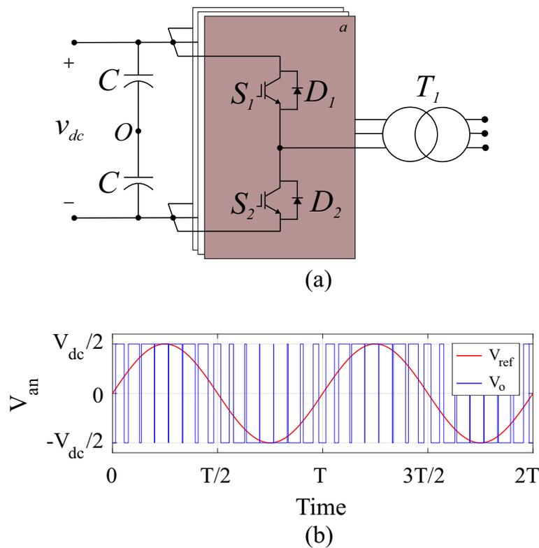
Figure 2 – Two-level voltage source converter: (a) Schematic of the three-phase circuit; (b) Two-level output voltage.
