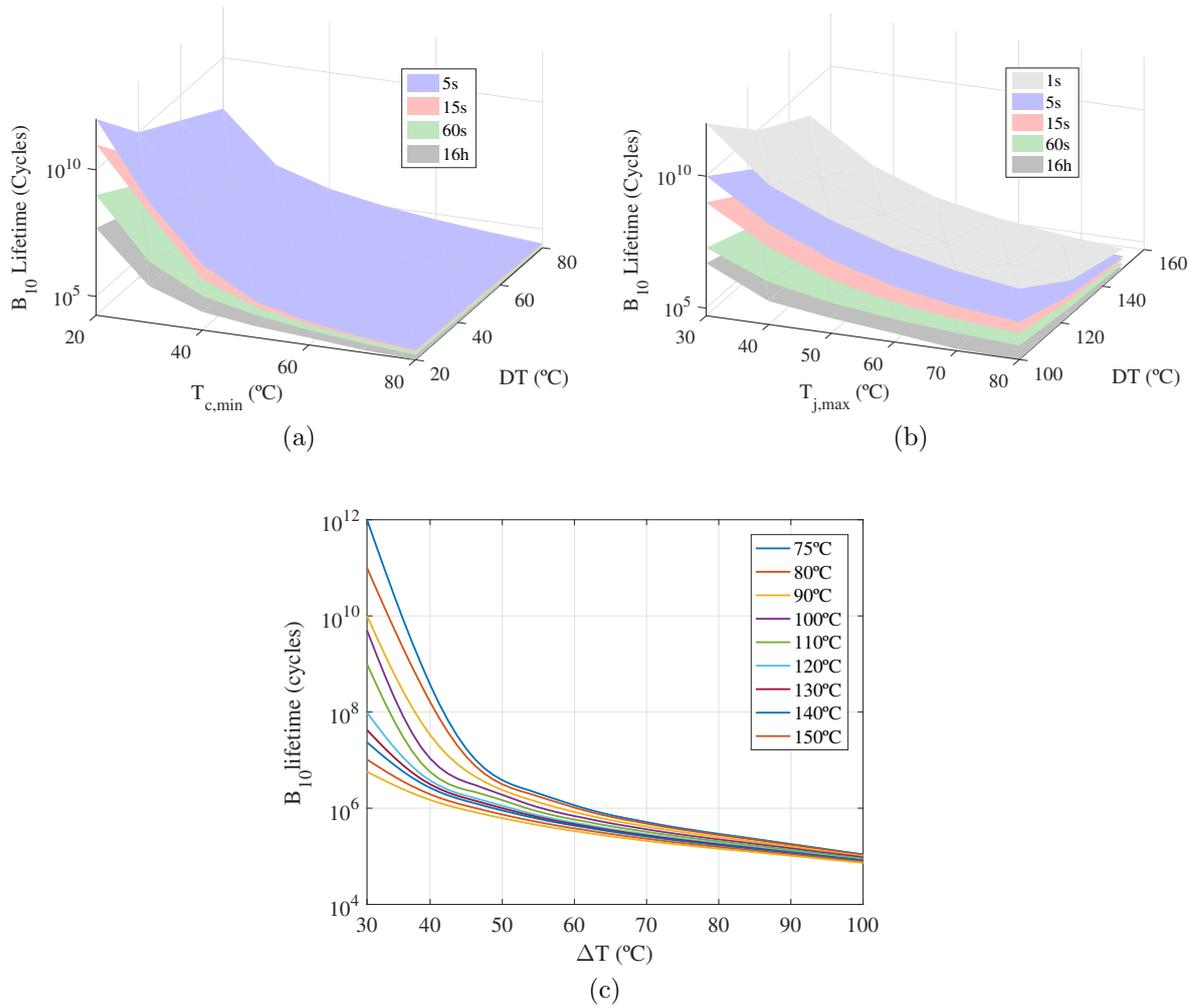
Figure 26 –  $B_{10}$  lifetime curves of Hipak IGBT module: (a) Baseplate solder; (b) Chip solder ; (c) Bondwire
