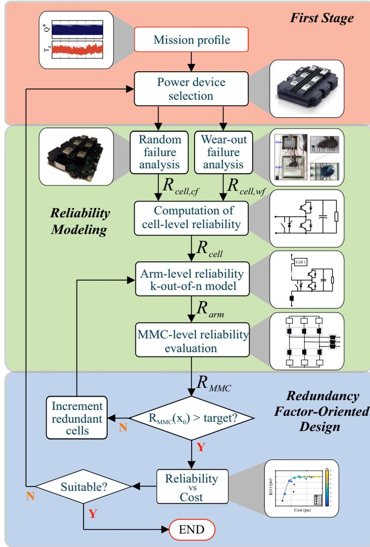
Figure 40 – Flowchart for the redundancy factor design.
