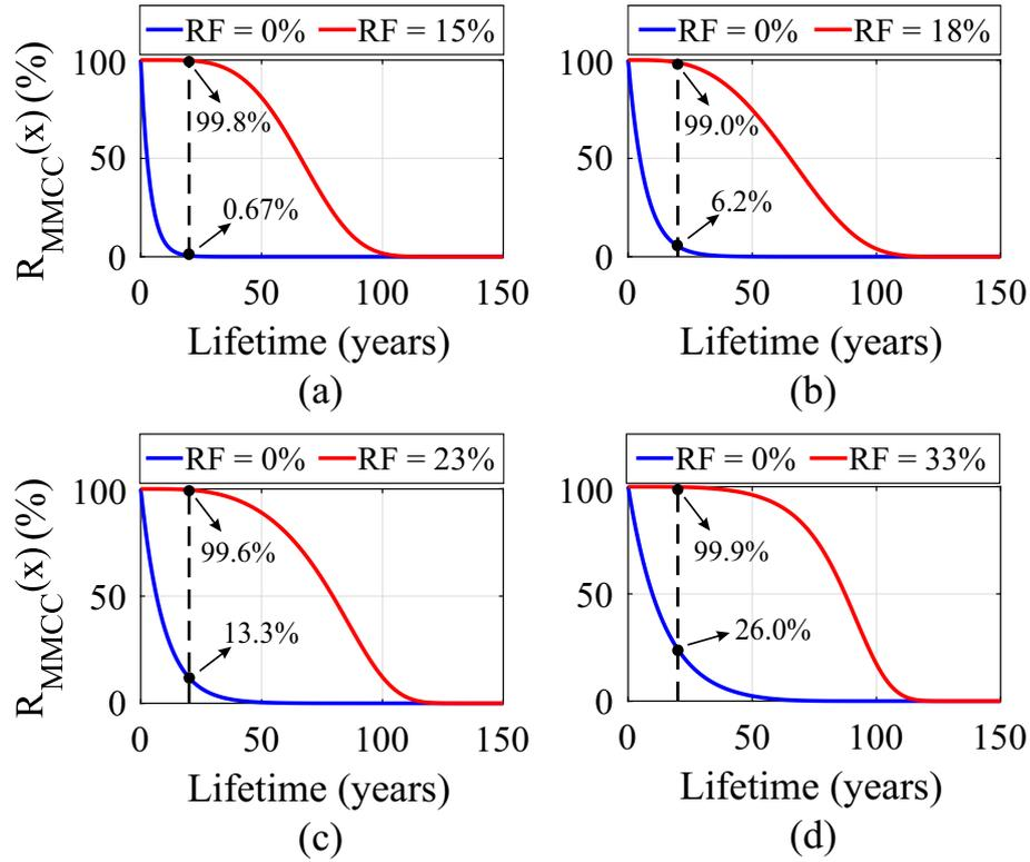
Figure 42 – MMCC system-level reliability function for 2 different redundancy factors: (a)  $C_{17}$ ; (b)  $C_{33}$ ; (c)  $C_{45}$ ; (d)  $C_{65}$ .
