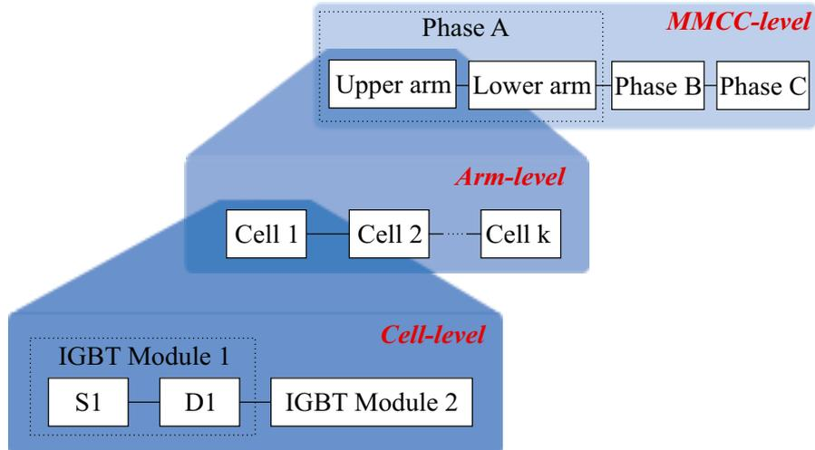
Figure 28 – System-level reliability block diagram of MMCC.
