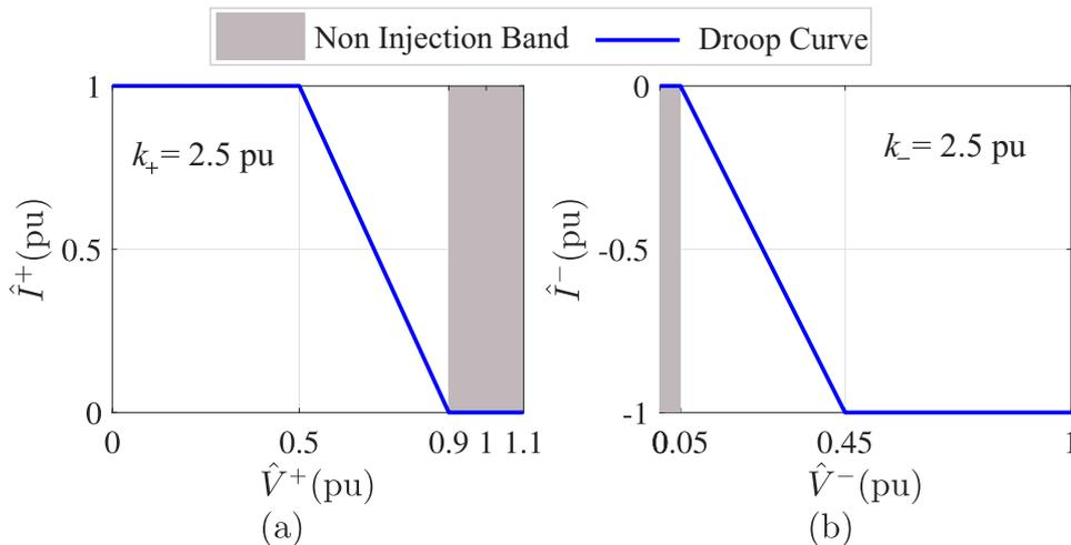
Figure 8 – Low voltage ride through current injection in Germany: (a) Positive sequence injection requirements; (b) Negative sequence injection requirements. Adapted from [VDE \(2015\)](#).
