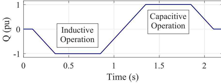
Figure 14 – Reactive power profile considering both inductive and capacitive operation.
