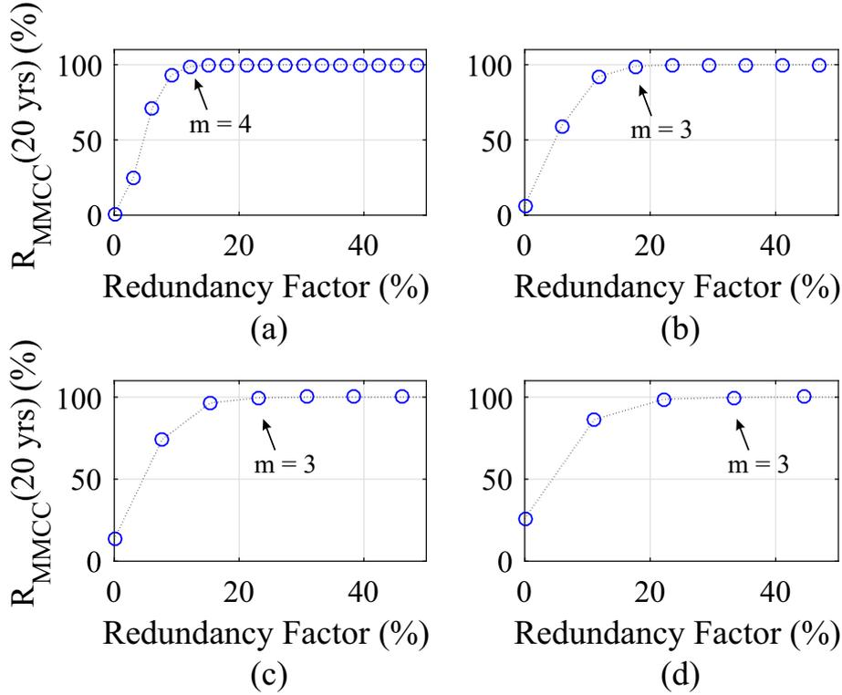
Figure 41 – MMCC system-level reliability at  $x_0 = 20$  years with different redundancy factors: (a)  $C_{17}$ ; (b)  $C_{33}$ ; (c)  $C_{45}$ ; (d)  $C_{65}$ .
