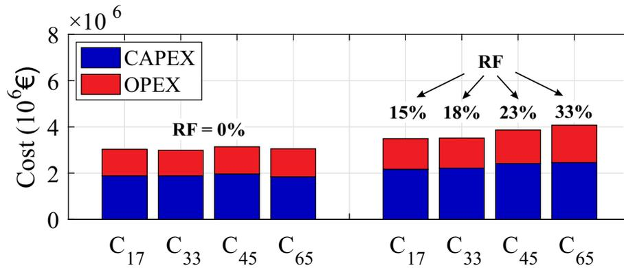
Figure 43 – Overall cost of all solutions divided into CAPEX and OPEX for 2 different redundancy factors.
