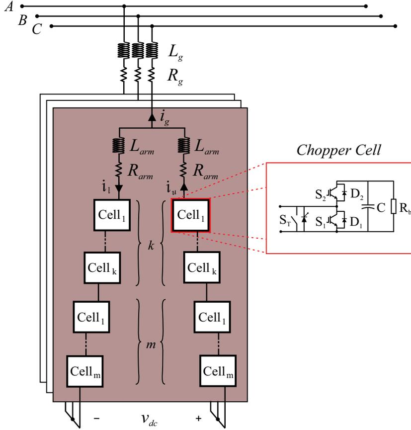
Figure 9 – Schematic of the DSCC-MMCC-based STATCOM.
