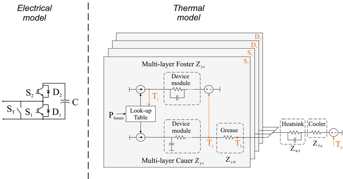
Figure 24 – Hybrid thermal model based on Foster and Cauer models with heatsink and cooling system.
