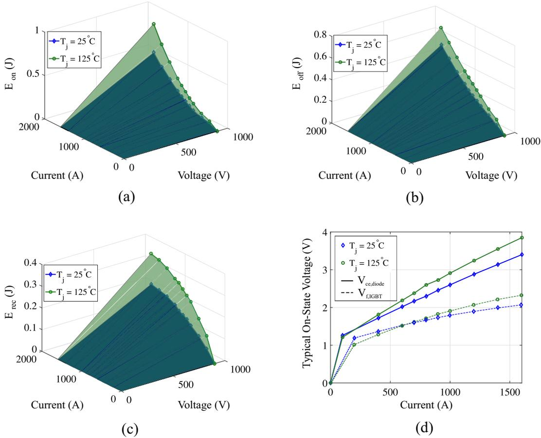
Figure 23 – Data extracted from a power module datasheet: (a) Turn-on switching energy (IGBT); (b) Turn-off switching energy (IGBT); (c) Reverse recovery energy (diode); (d) Typical IGBT on-state characteristics and diode forward characteristics. In this example, the part number 5SND 0800M170100 is considered.
