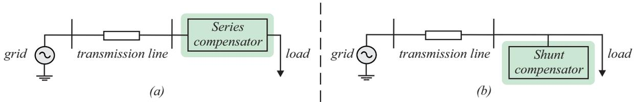
Figure 1 – Schematic of FACTS controllers for reactive power compensation: (a) series compensation; (b) shunt compensation.
