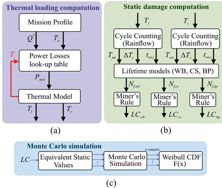
Figure 22 – Wear-out analysis flowchart: (a) Translation of the mission profile into thermal stresses; (b) Static damage computation through reliability model; (c) Monte Carlo simulation for computation of component and system-level reliability.
