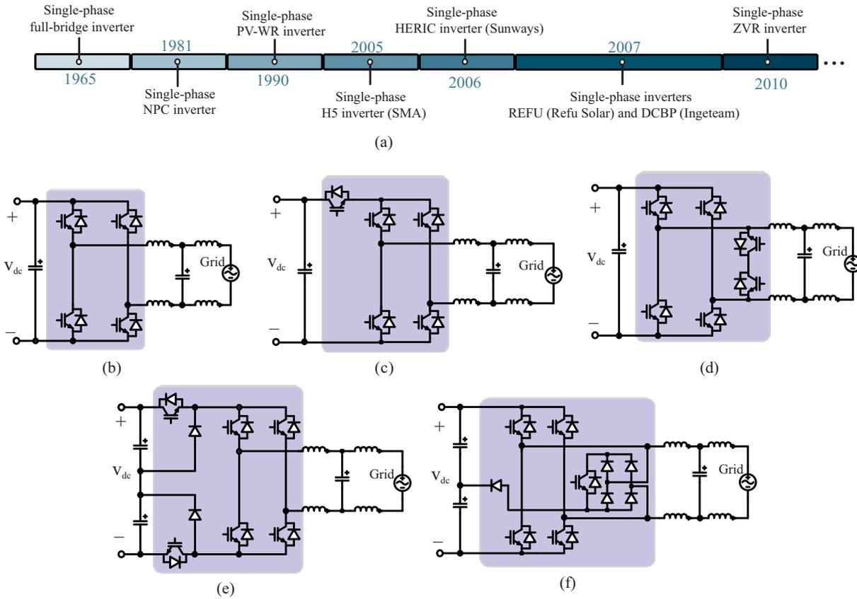
Figure 1 – (a) Summarized timeline of two-level full-bridge transformerless inverter topology developments. (b) Classical FB topology, (c) H5 topology, (d) HERIC topology, (e) DCPB topology and (f) ZVR topology.
