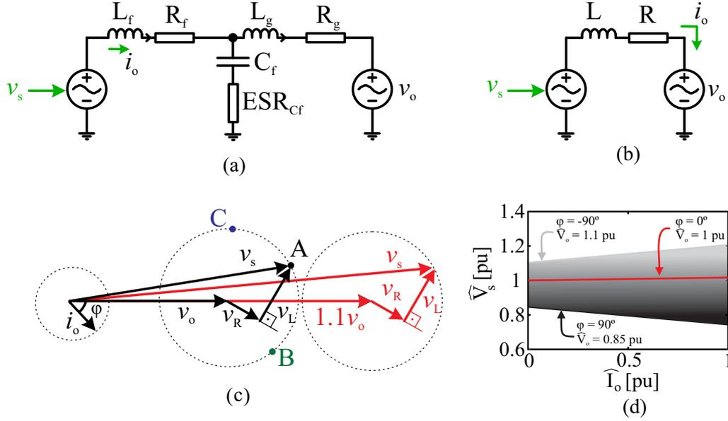
Figure 10 – (a) Average model of the single-phase PV system. (b) Simplified average model of the single-phase PV system, using the Padé approximant approach. (c) Simplified phasor diagram of the converter, considering different grid voltage and  $\varphi$  scenarios. (d) Range of synthesized voltage by the converter required to remain grid-connected, as a function of the injected current,  $\varphi$  and grid voltage ( $S_b = 3300$  VA and  $V_b = 311$  V).
