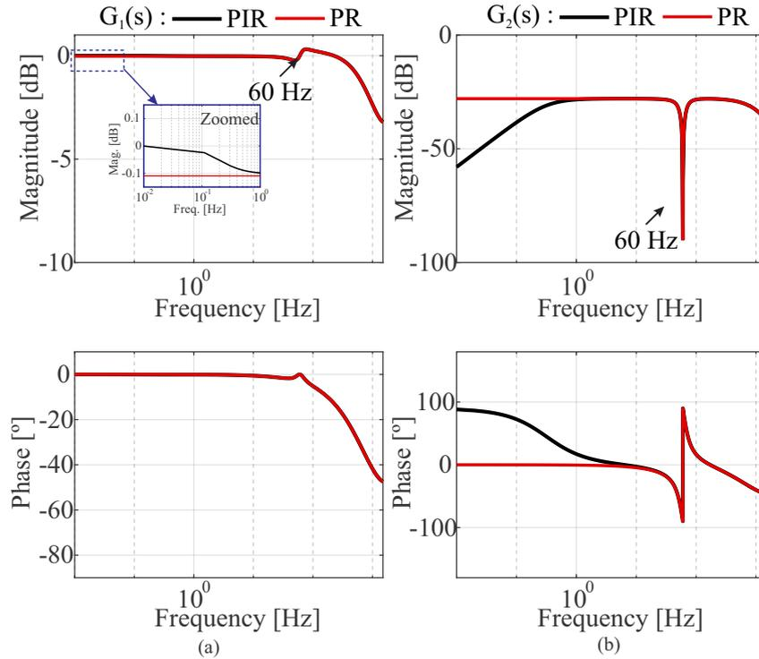
Figure 33 – Closed-loop Bode diagram of the compensated system with PR and PIR: (a) Magnitude and phase of  $G_1(s)$ . (b) Magnitude and phase of  $G_2(s)$ .
