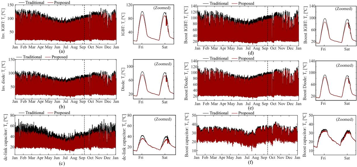
Figure 39 – Junction temperature and hot-spot temperature: (a) inv. IGBT, (b) inv. diode, (c) de-link capacitor, (d) boost IGBT, (e) boost diode and (f) boost capacitor.
