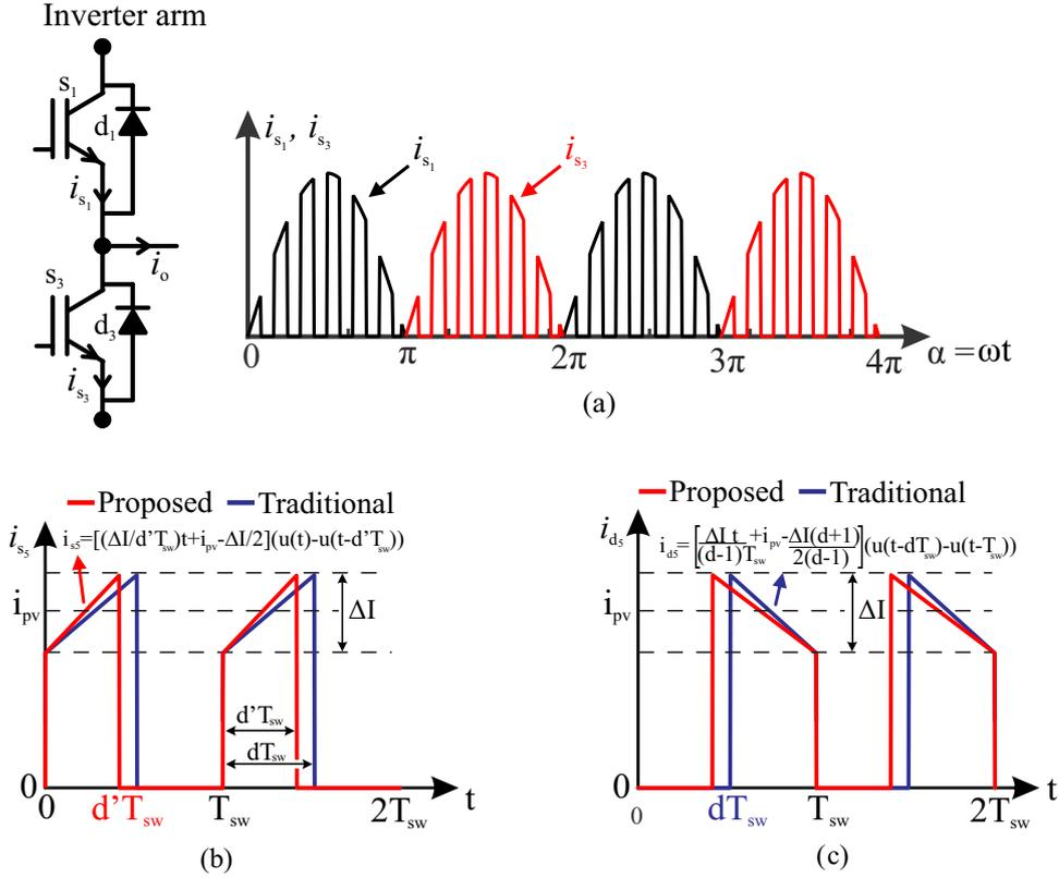
Figure 12 – (a) IGBT typical collector current waveforms. Typical current waveforms considering traditional operation (dc-link voltage set at  $v_{dc}^*$ ) and minimum dc-link voltage operation, for boost (a) IGBT and (b) diode.
