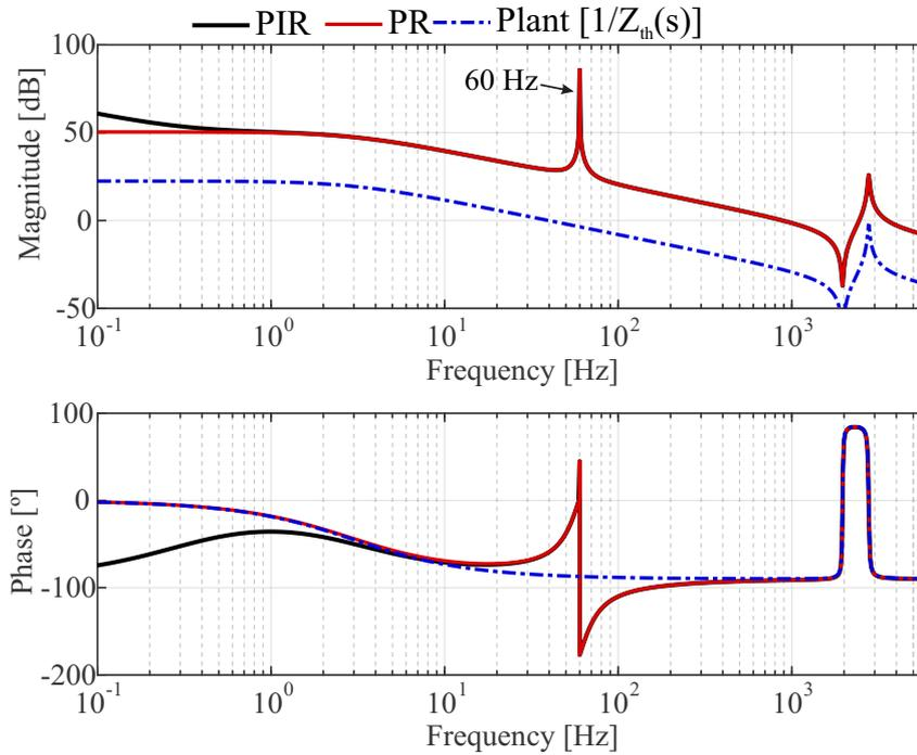
Figure 32 – Open-loop Bode diagram of the non-compensated system and compensated with PR and PIR: (a) Magnitude. (b) Phase.
