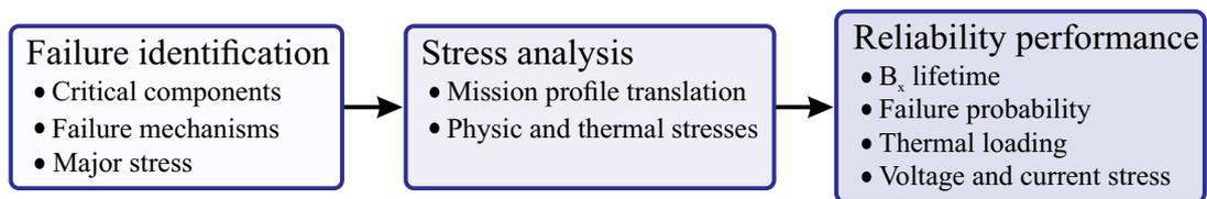
Figure 15 – Flowchart diagram to assess the PV inverter reliability performance.
