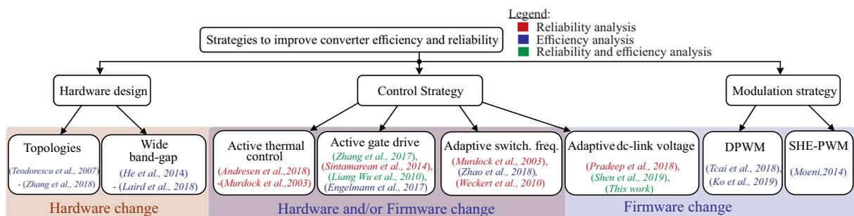
Figure 3 – Overview of strategies proposed to improve static converters efficiency and reliability in the literature.
