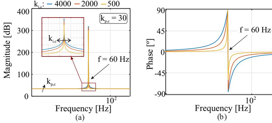
Figure 9 – (a) Magnitude and (b) phase response of the PR-controller for different  $k_{i,c}$ .
