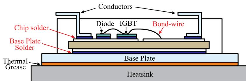
Figure 16 – Structure of a cross section of standard power device.
