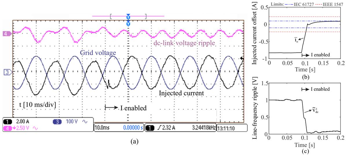
Figure 34 – (a) Cascade-control dynamic performance of single-phase PV inverter when the proposed dc-component mitigation strategy is enabled.  $v_o$  [100 V/div];  $i_o$  [2 A/div];  $v_{dc}$  ripple [2.5 V/div] and time [10 ms/div]). Corresponding dynamics result when the PIR controller is enabled: (b) Current dc-component injection. (c) Line-frequency ripple amplitude of the dc-link voltage.
