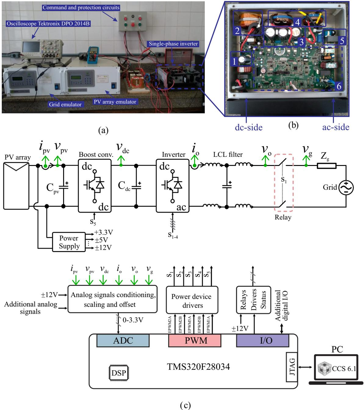
Figure 26 – (a) Experimental setup. (b) PV inverter components: 1) boost capacitor, 2) boost inductor, 3) dc-link capacitor bank, 4) filter inductors, 5) filter capacitor, 6) conditioning electronic circuits. (c) Schematic of connection between hardware and DSP.
