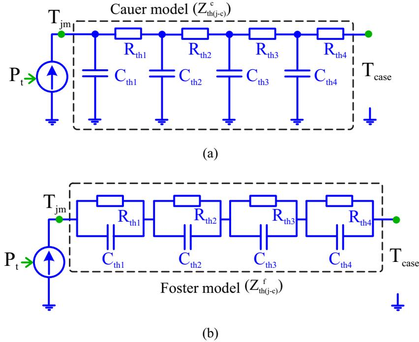
Figure 19 – Thermal impedance models: (a) Cauer-model. (b) Foster-model.
