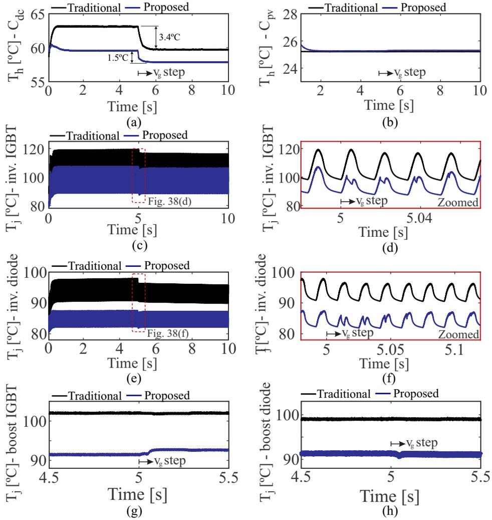
Figure 38 – Simulated temperature dynamics of reliability-critical components after system disturbance application, at 5 s. Hot-spot temperature of (a) dc-link and (b) boost capacitors. (c) Inverter IGBT junction temperature and (d) its transient zoom. (e) Inverter diode junction temperature and (f) its transient zoom. Junction temperature of (g) boost IGBT and (h) boost diode.
