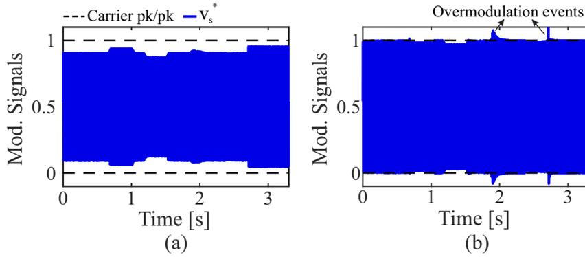
Figure 36 – Synthesized voltage reference and modulator carrier peak-to-peak during voltage and power steps: (a) Fixed dc-link voltage strategy. (b) Minimum dc-link voltage strategy.
