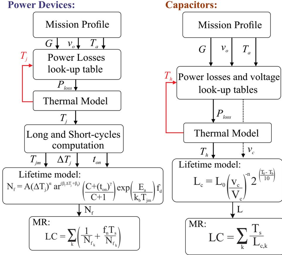
Figure 22 – Flowchart for the reliability evaluation of power devices and capacitors.
