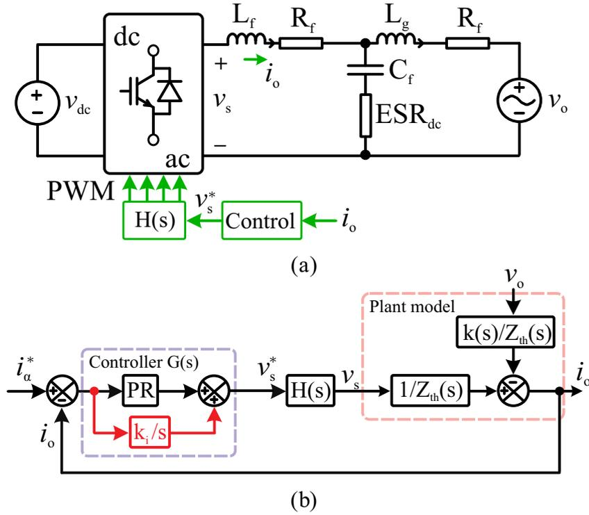
Figure 31 – (a) Diagram of a typical single-phase PV system. (b) Closed loop of current control architecture, modeled with delay due to sampling and PWM scheme.
