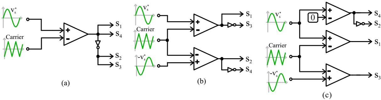
Figure 7 – (a) Bipolar, (b) unipolar and (c) hybrid modulation structures.
