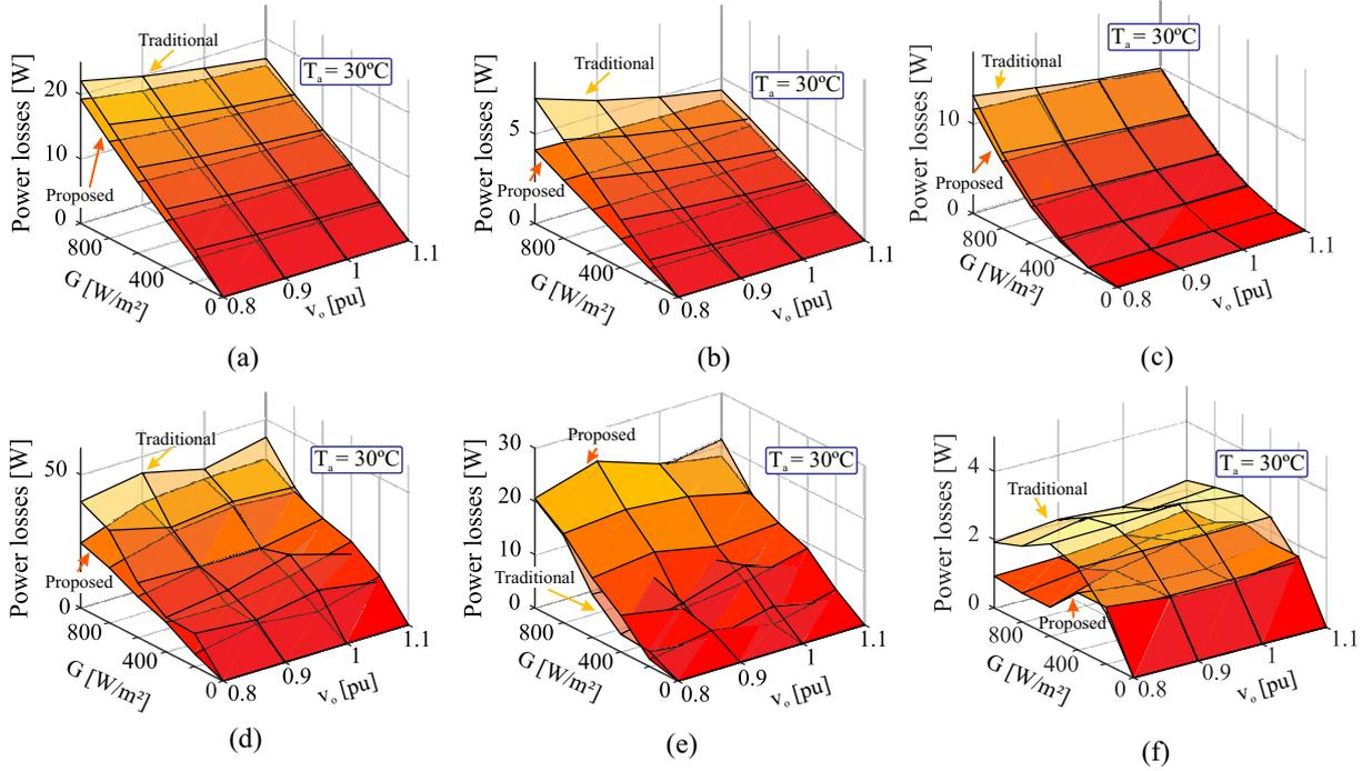
Figure 21 – Power devices and al-caps total losses, considering different solar irradiance and grid voltage conditions: (a) Inv. IGBTs and (b) inv. diodes. (c) Dc-link capacitor (partnumber B43630C5397M0 from TDK). (d) boost IGBT and (e) boost diode. (f) Boost capacitor (partnumber B43630C5397M0 from TDK).
