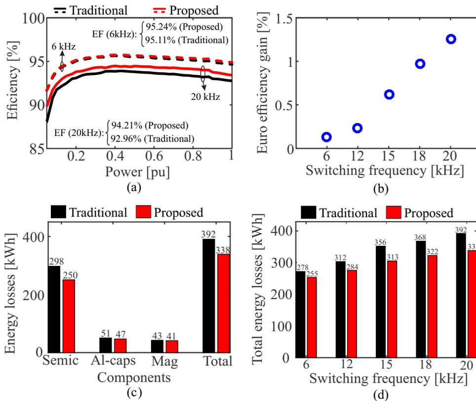
Figure 42 – (a) Converter efficiency for  $f_{sw} = 6$  kHz and 20 kHz, considering the proposed and traditional control strategies. (b) Euro efficiency gain for the converter switching at 6, 12, 15, 18 and 20 kHz. (c) PV inverter energy losses with  $f_{sw} = 20$  kHz, separated by components and evaluated during 1-year mission profile. (d) Total energy losses considering the switching frequency equal to 6, 12, 15, 18 and 20 kHz.
