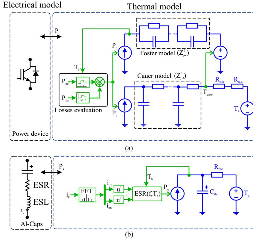
Figure 20 – Simplified thermal model of (a) power devices and (b) al-caps, from the electrical domain to thermal domain linked by power losses.
