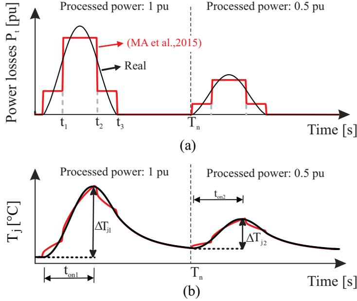
Figure 23 – Pulsed losses in power devices: (a) real loss and approximate loss by a sum of two-square pulses. (b) Corresponding real and approximate junction temperature.
