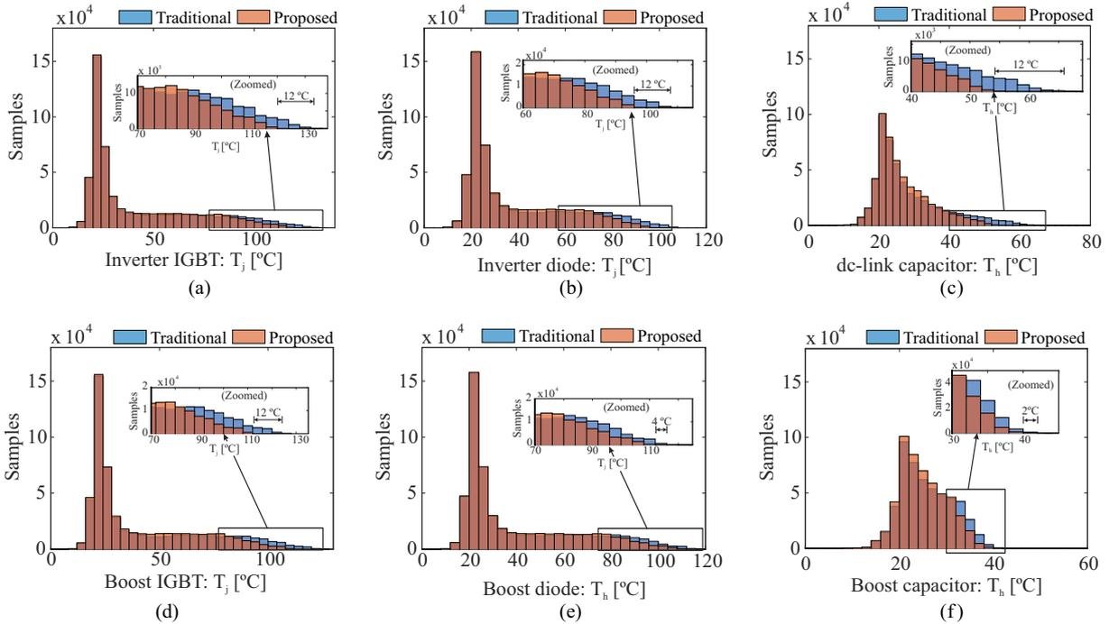
Figure 40 – Junction temperature and hot-spot temperature histograms for all 1-year MP samples translated to thermal loading (5,256,000 samples): (a) inv. IGBT, (b) inv. diode, (c) de-link capacitor, (d) boost IGBT, (e) boost diode and (f) boost capacitor.
