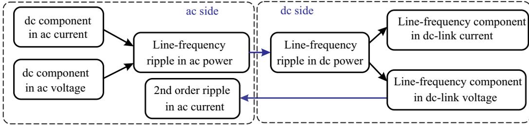
Figure 29 – Dc-component effect on single-phase PV systems.
