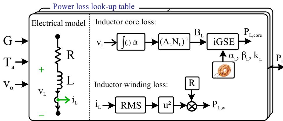
Figure 25 – Procedure for assembling the core and windings loss look-up table of magnetic components.
