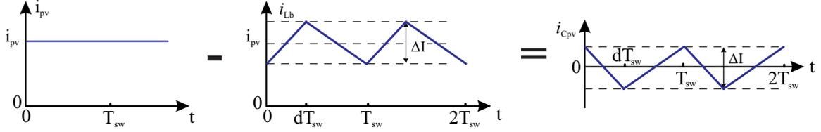
Figure 13 – Typical boost capacitor current waveform, composed of the current drained from the PV array and the boost inductor current.
