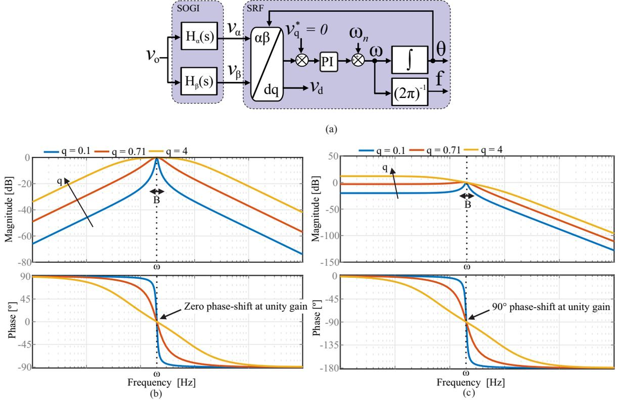
Figure 6 – (a) Block diagram SOGI-PLL structure. Frequency response of the closed-loop transfer function of (b)  $H_\alpha(s)$  and (c)  $H_\beta(s)$ .
