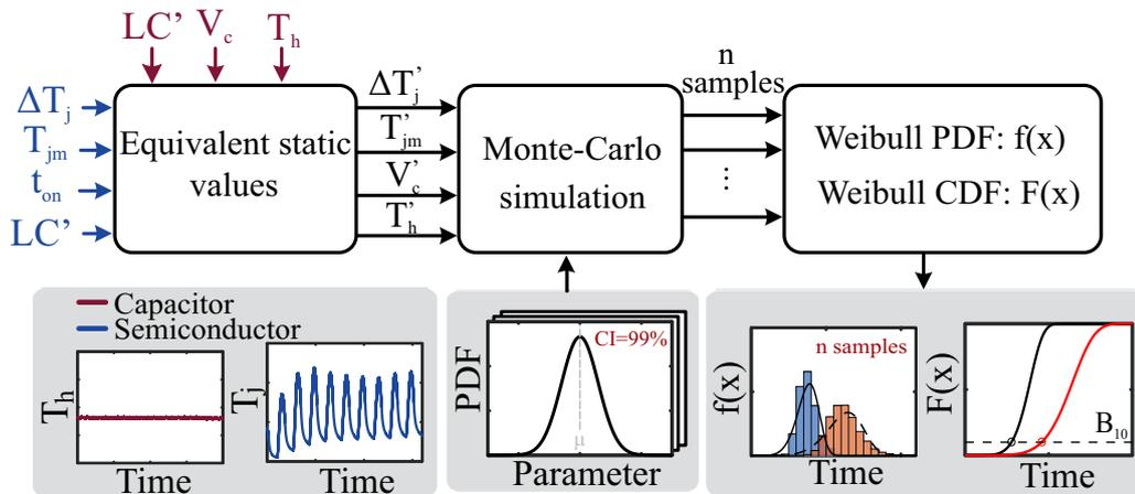
Figure 24 – Flowchart of Monte-Carlo simulation for power devices and capacitors.
