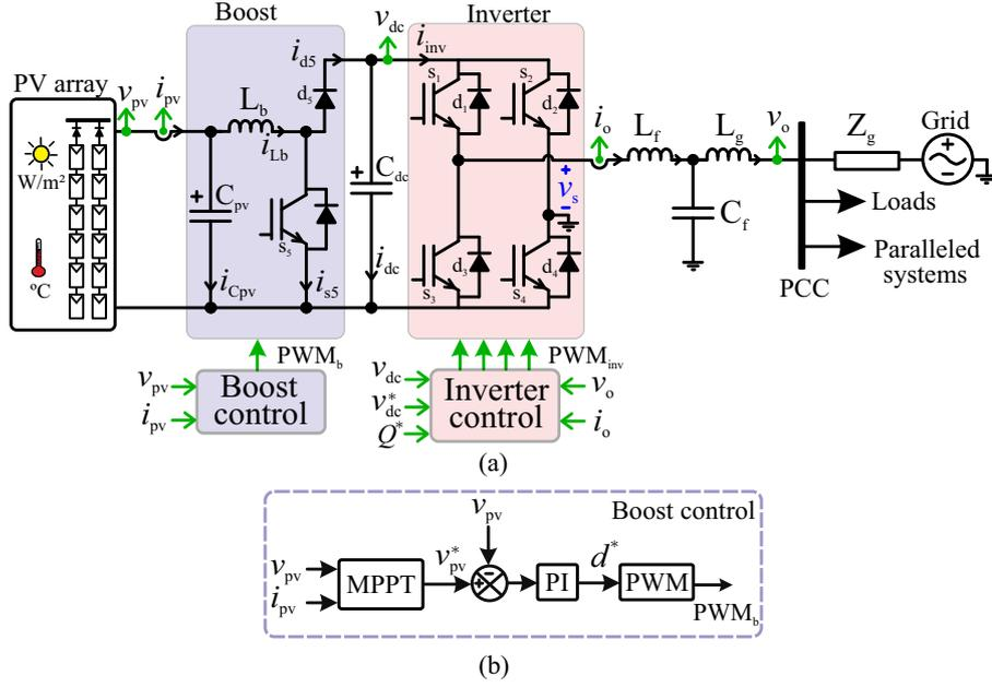
Figure 5 – (a) Schematic of a two-stage single-phase grid-connected PV system. (b) Boost converter control block diagram.
