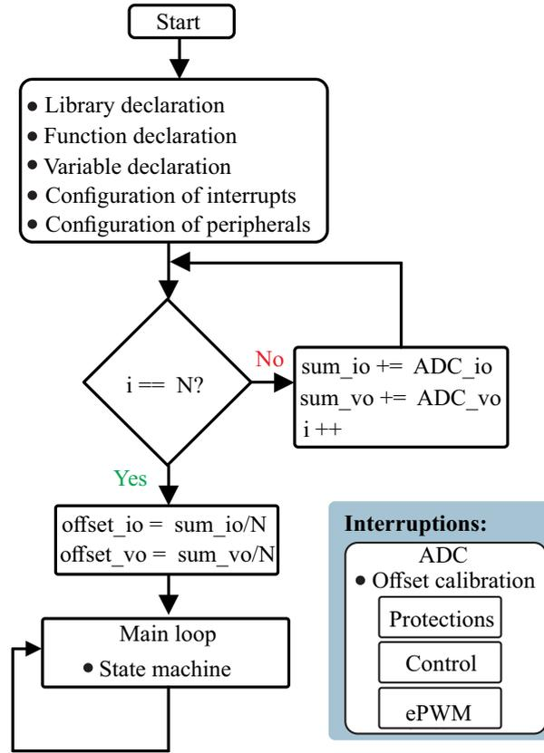
Figure 30 – Flowchart of the offset mitigation algorithm caused by the measurement biases of the ac sensors.
