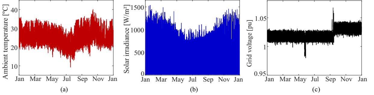
Figure 18 – One-year mission profile of: (a) solar irradiance, (b) ambient temperature and (c) grid voltage.
