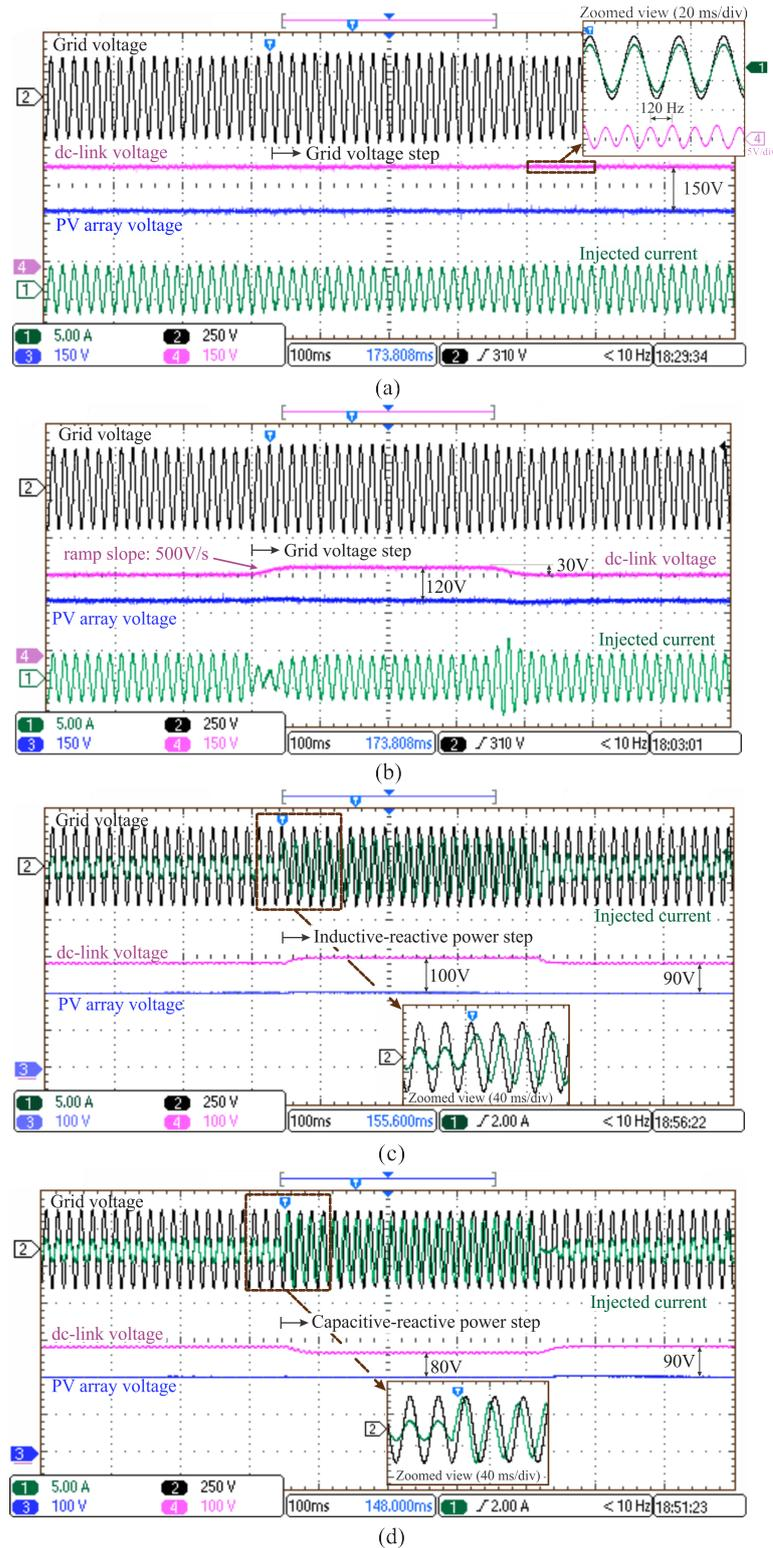
Figure 37 – Experimental results of the two-stage grid-connected PV inverter (grid voltage [250 V/div]; injected current [5 A/div]; dc-link voltage [150 V/div], PV array voltage [150 V/div] and time [100 ms/div]). (a) Fixed and (b) minimum dc-link voltage operation when a 10% grid overvoltage variation is applied. Minimum dc-link voltage operation when an (c) inductive- and (d) capacitive-reactive power step is performed.
