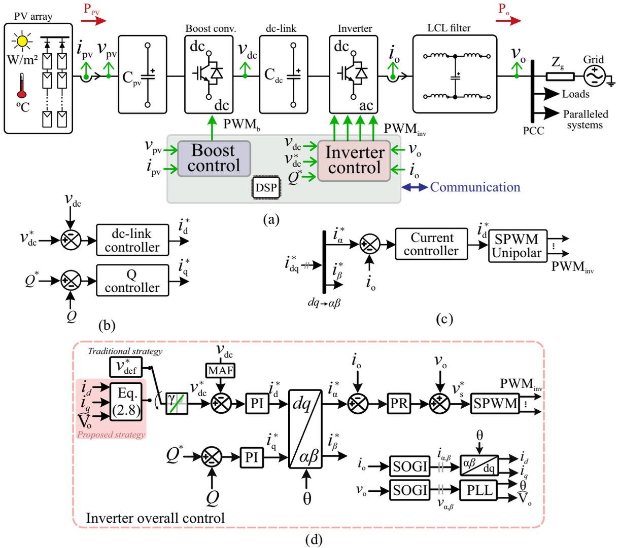
Figure 8 – Typical configurations and control structures of single-phase grid-connected PV systems. (a) Hardware overview. (b) Inner control loop in  $\alpha\beta$ -reference frame. (c) Outer control loop for two-stage PV systems in  $dq$ -reference frame (d) Complete inverter cascade-control structure.
