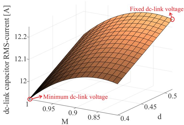
Figure 14 – RMS-current stress evaluation of the dc-link capacitor bank according to the modulation index and duty-cycle operating ranges between the minimum and fixed dc-link voltage (setup parameters are used under rated power).
