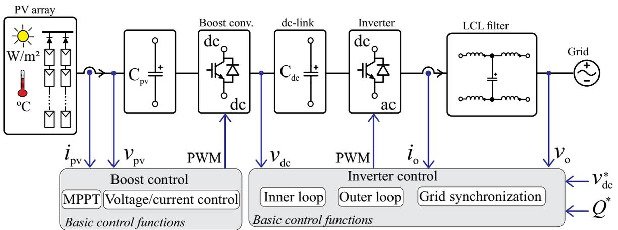
Figure 2 – Structure and main control functions of a typical two-stage single-phase grid-connected PV system.
