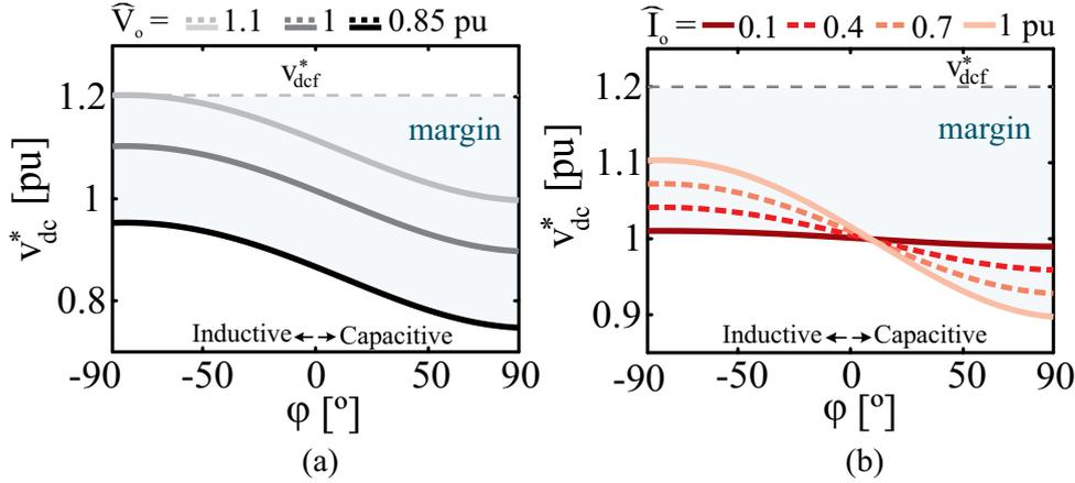
Figure 11 – Adaptive dc-link voltage reference according to model (2.7) as a function of the converter operating angle, considering (a) rated fixed current injection and (b) grid voltage set at 1 pu (filter impedance equal to  $0.01 + j0.1$  pu).
