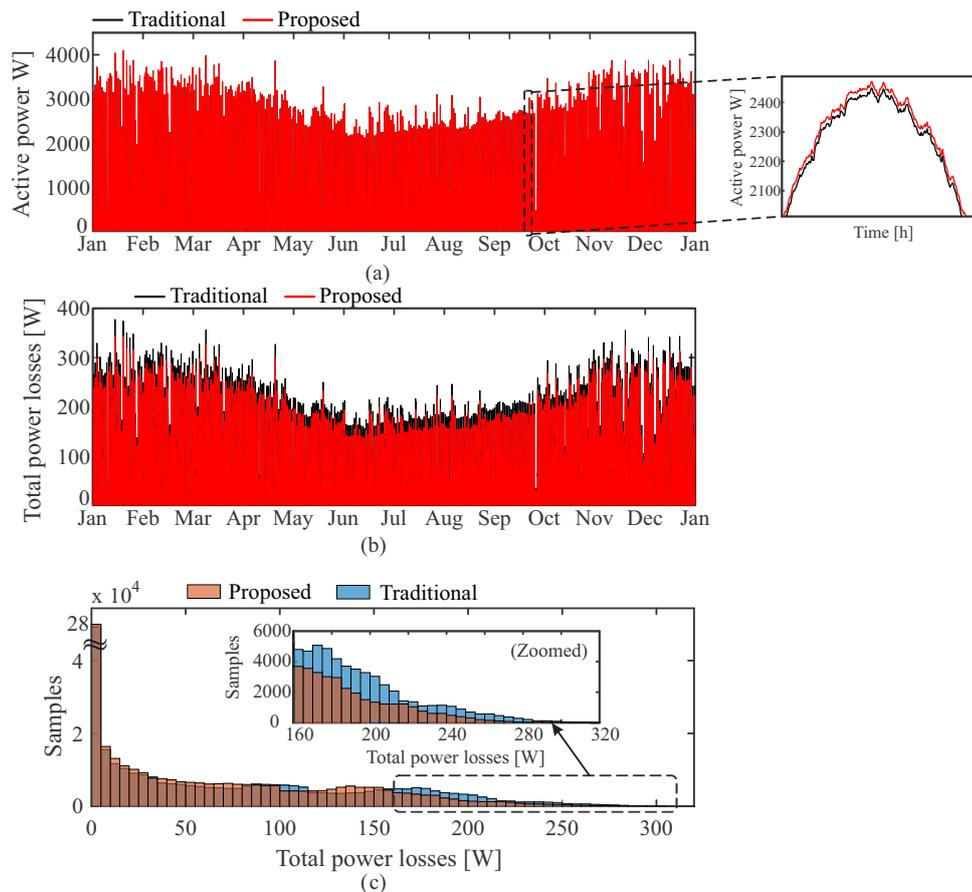
Figure 41 – (a) Active power at the inverter output injected in the grid after computing the component losses, for the proposed and traditional strategies. (b) Sum of power loss contributions from semiconductors, al-caps and magnetic devices, for the proposed and traditional strategies. (c) Power losses histogram of all inverter components for 1-year MP samples (5,256,000 samples).
