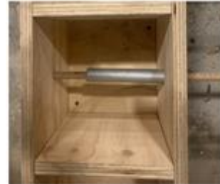
d) Steel conduit used as bond breaker.
