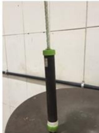
c) Caps used to ensure GFRP bar alignment on the steel tube.
