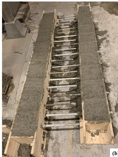
Figure 5.2 – ASTM D7913 test specimens after concrete casting at (a) CEFET-MG and (b) PITT.
