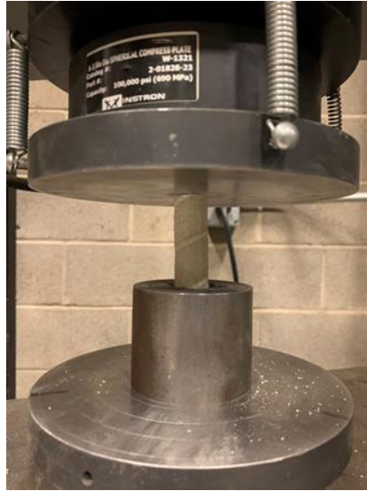
d) #5 bar being tested – bar is pushed into steel cylinder, shearing off sand coating
