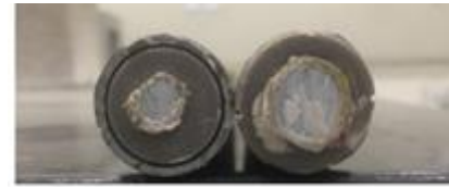
b) Bars anchored with steel tube.
