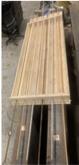
a) Prism forms prior concrete casting.
