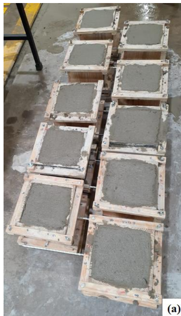
Figure 5.2 – ASTM D7913 test specimens after concrete casting at (a) CEFET-MG and (b) PITT.
